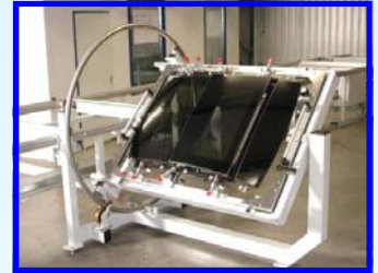
Turning module in "inventor" and as produced The shown product carriers of approx. 1400 x 1800 mm are not the maximum size that IPA can handle.
